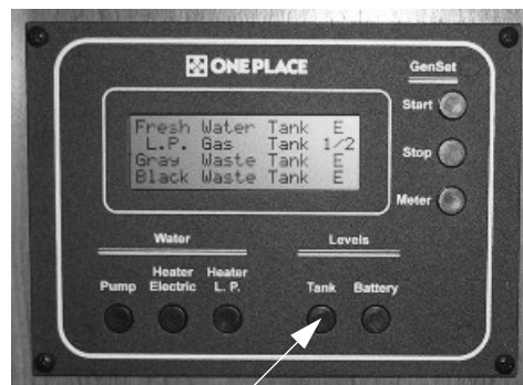
Tank Levels Switch
