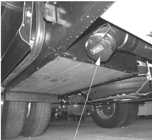
Sewage Drain Outlet (Located underneath coach behind driver side rear wheel) -Typical View
