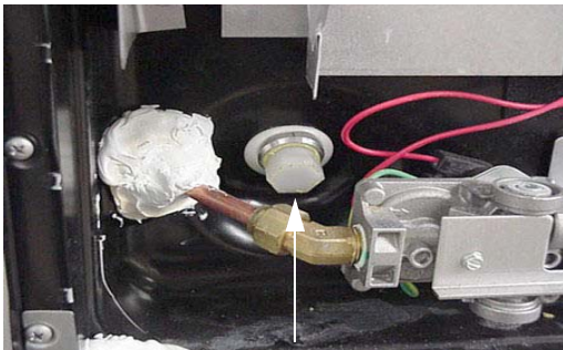
Water Heater Drain Plug (Remove with socket)
