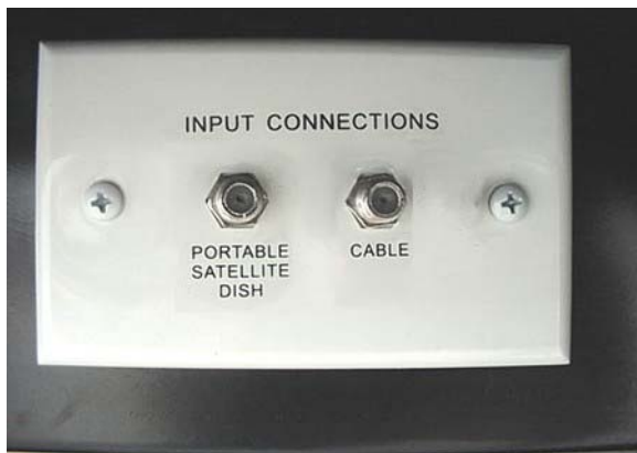
Exterior Cable TV and Satellite Connections (Located in shoreline or utility compartment, depending on model)
