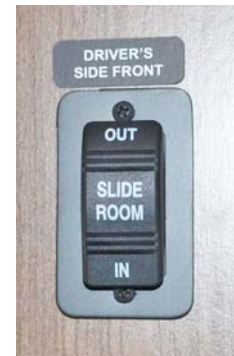
Slideout Switch (Your coach may have one or more slideout switches depending on model, options, and available equipment) -Typical View
