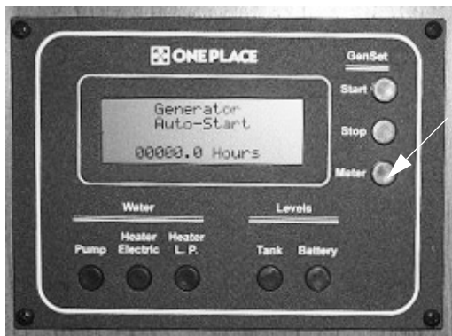
Generator Hourmeter Button -Typical View
