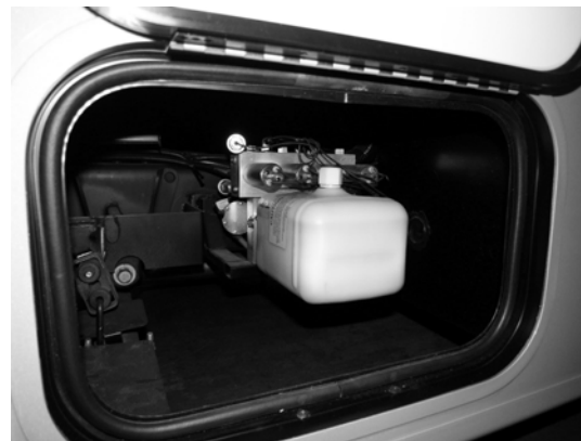
Hydraulic Oil Reservoir (Located in mid-passenger side compartment) -Typical View
