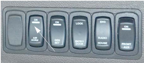
Air Horn Switch (Located on dash or driver side trim panel) -Typical View
