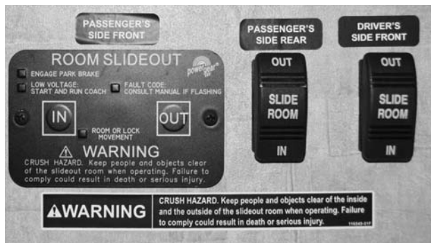
Slideout Switches (Your coach may have one or more of these switches depending on model, options, and available equipment) -Typical View
