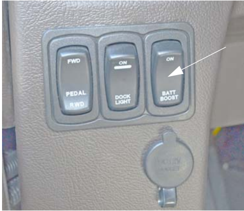
Battery Boost Switch (Located on dash)
