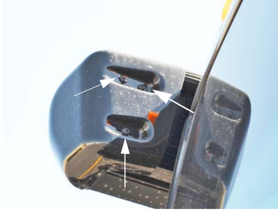
Entry Door Awning End Cap (Located on front inward end of Entry Door Awning)
