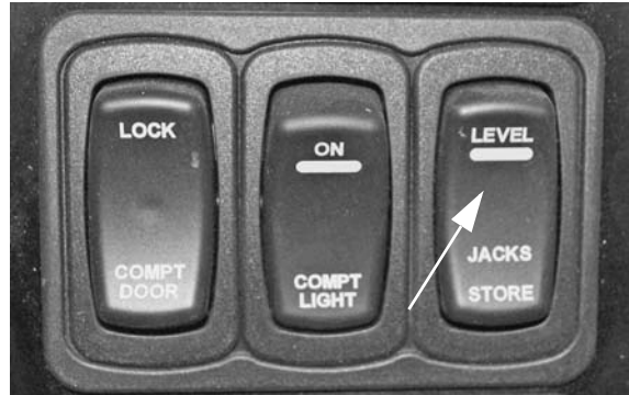
Auto Level Remote Switch (Located near entrance door) -Typical View
