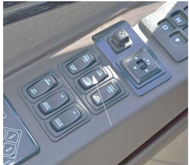
Tag Axle Switch (Located on the driver side trim panel) -Typical View
