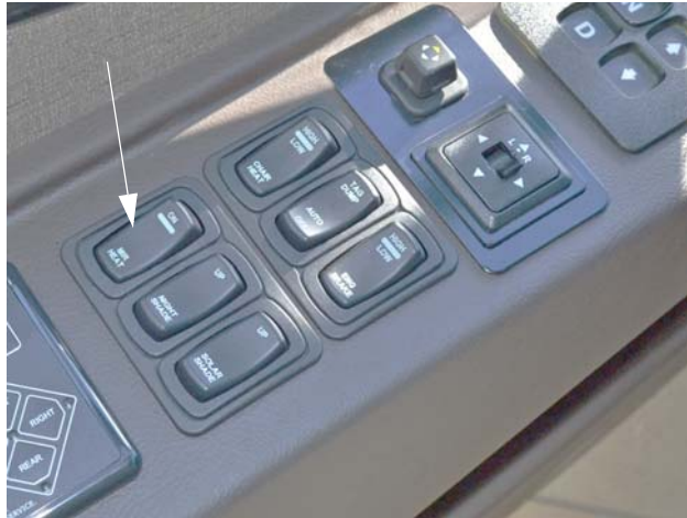
Mirror Heater Switch (Located on driver side trim panel) -Typical View
