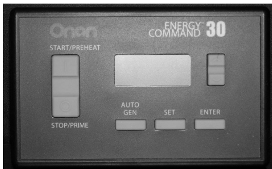
AGS Control Pad (Located near monitor panel)
