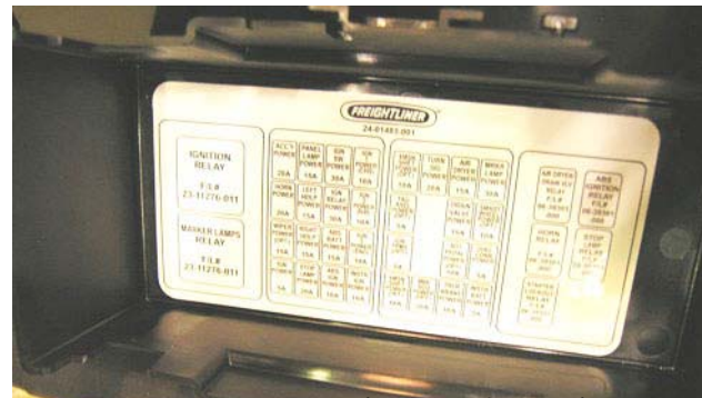
Fuse Diagram (inside of cover)
