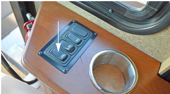
Step Cover Switch (Located on passenger side armrest) -Typical View
