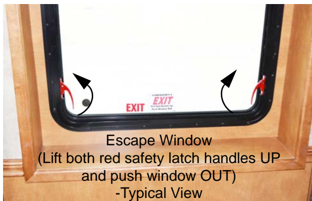
Escape Window (Lift both red safety latch handles UP and push window OUT) -Typical View
