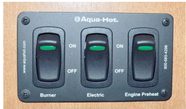
Hydronic Heating System Interior Control Switches (Located near monitor panel) -Typical View
