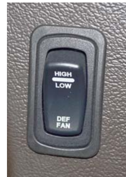
Defrost Fan Switch (Located on dash) -Typical View
