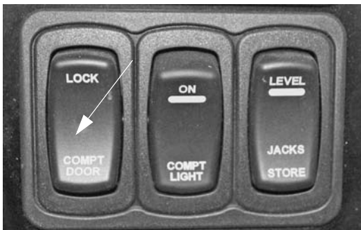
Power Door Locks - Compartment Doors (Located on entry switch panel) -Typical View
