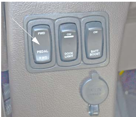
Adjustable Pedal Switch (Located on dash) -Typical View
