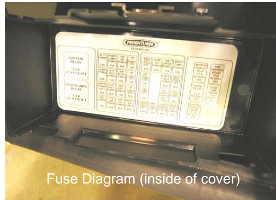
Automotive Fuses (cover removed)
