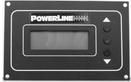
PCS Display Panel (Located near monitor panel) -Typical View
