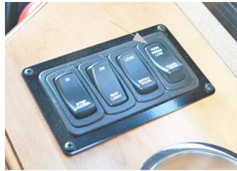
Chair Heat Switch (Located on driver and passenger side trim panels)
