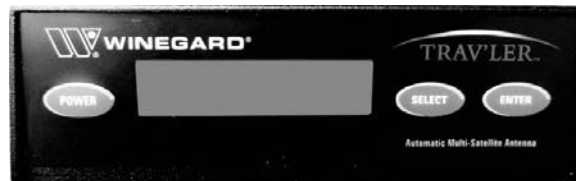
Automatic Multi-Satellite Dish Control (Located in overhead cabinet or entertainment center cabinet, depending on model) -Typical View
