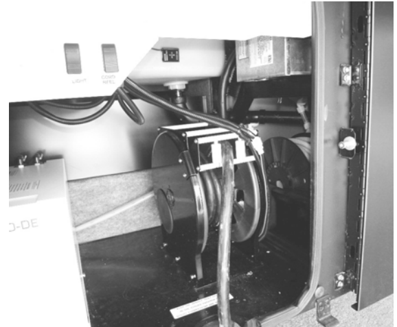
Power Cord Reel (Located inside an exterior compartment) -Typical View
