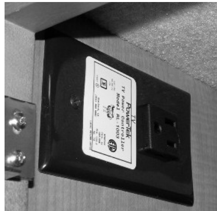
Front TV Ignition Switch Interlock -Typical View
