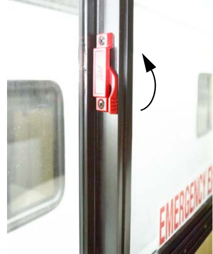
Slider Window Latch (Lift latch UP and slide window open) -Typical View
