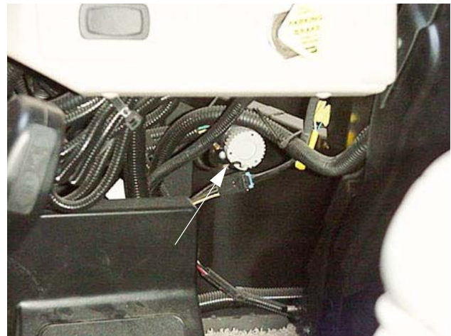
Diagnostic Plug (Located on steering column support beneath left side of dash) -Typical View
