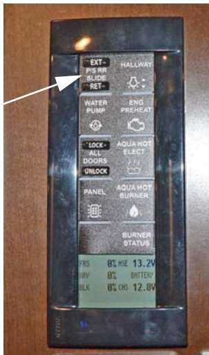
Rear Slideout Switch (Your coach may have one or more of these switches depending on model, options, and available equipment) -Typical View
