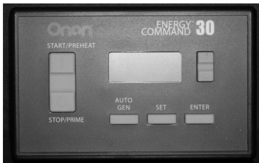
AGS Control Pad (Located near monitor panel)
