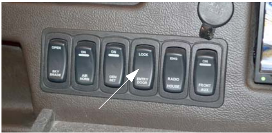
Power Door Locks - Entry Door (Located on dash) -Typical View
