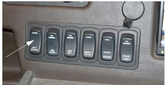
Skylight Shade Control Switch (Located on dash)
