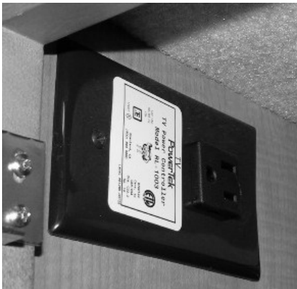
Front TV Ignition Switch Interlock -Typical View
