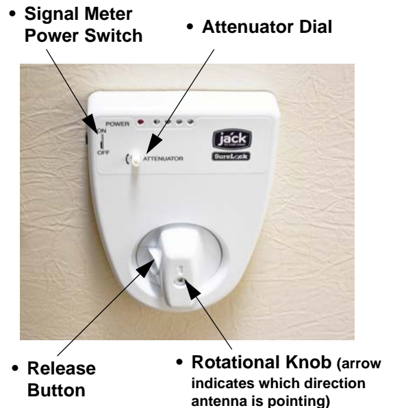
Digital Antenna Signal Meter (Located on ceiling)
