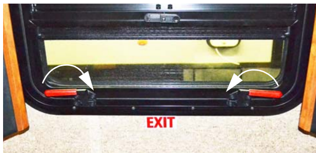
Escape Window (Lift both red safety latch handles UP and push window OUT) -Typical View
