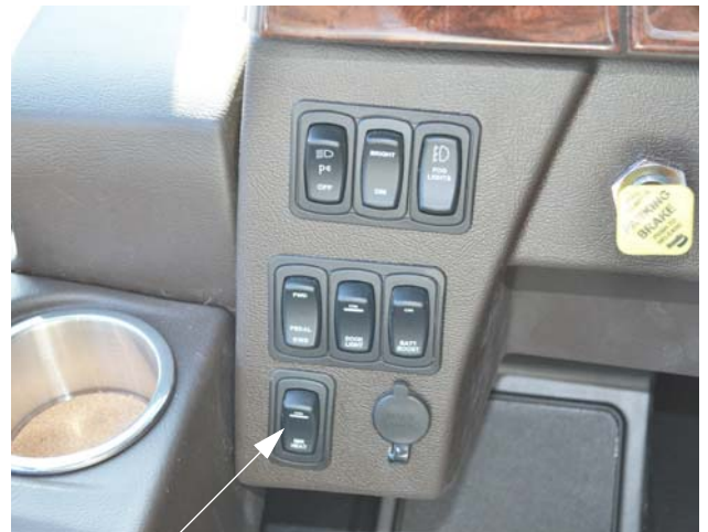
Mirror Heater Switch (Located on dash) -Typical View
