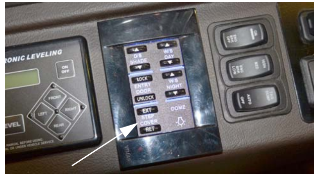
Step Cover Switch (Located on driver side trim panel) -Typical View
