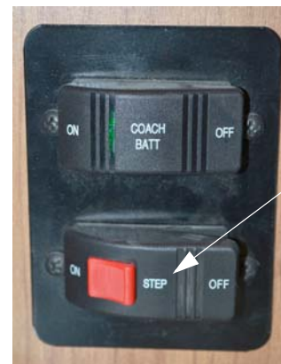
Entry Step Switch (Located near entrance door) -Typical View
