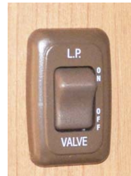
LP Tank Valve Switch
