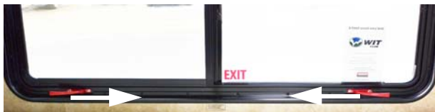
Escape Window (Pull both latch handles inward and push window open) -Typical View
