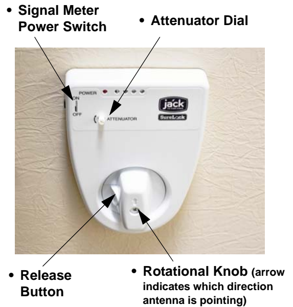
Digital Antenna Signal Meter (Located on ceiling)
