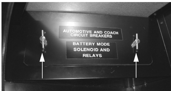
Automotive Chassis and House 12-Volt Circuit Breakers (Located in passenger side compartment) * Turn latches to remove cover
