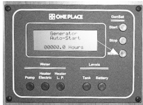
Generator Hourmeter Button -Typical View
