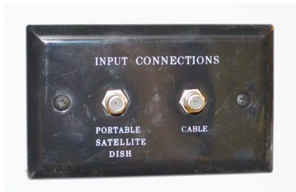
Exterior Cable TV and Satellite Connections (Located in shoreline or utility compartment, depending on model)
