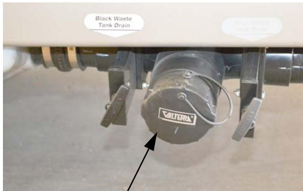
Sewage Drain Outlet (Located on the underside of water service center) -Typical View
