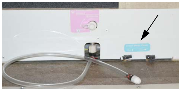
Waterline Drain Valve
