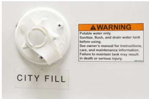
Fresh (City) Water Inlet -Typical View
