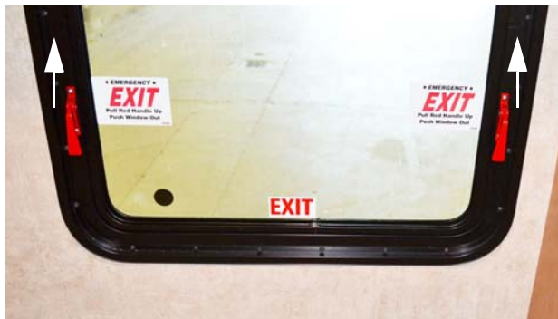
Escape Window Pull Red Handles Up and Push Window Out. -Typical View
