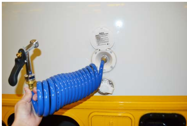
Exterior Shower/Wash Station -Typical View
