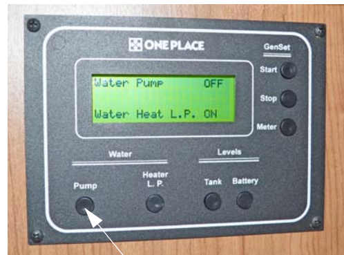
Water Pump Switch
