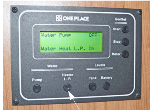
LP Gas Water Heater Switch
