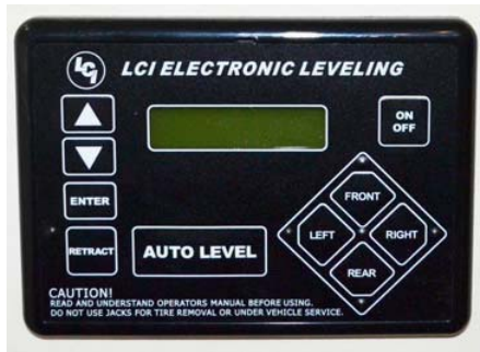
Leveling System Control Panel (Located on dash)
