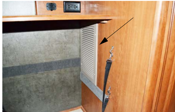
Water Supply Faucets (Located behind vent along side the Stackable Washer/Dryer cabinet near inTable storage location) * Model 32D shown
