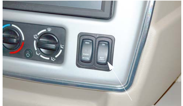
Passenger Side Map Light Switch (Located on dash)
