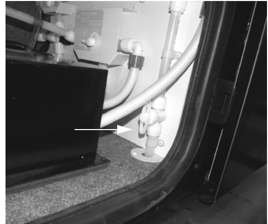
Waterline Drain Valve - Typical Installation
