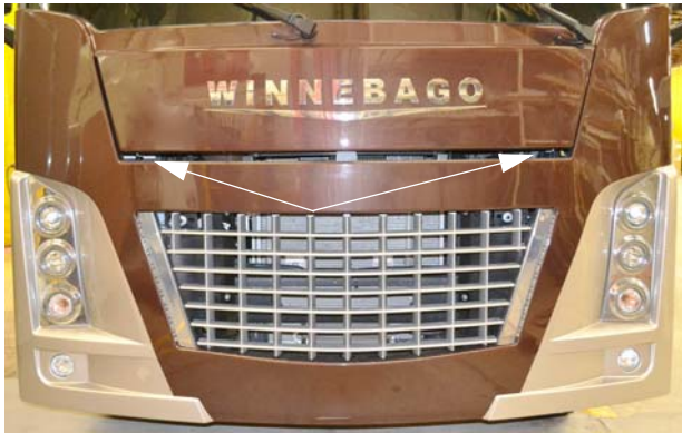
Hood Latches (Pull down to release the latches)
