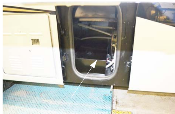
Water Pump (Located inside a passenger side compartment in front of water heater) * Models 32D shown
