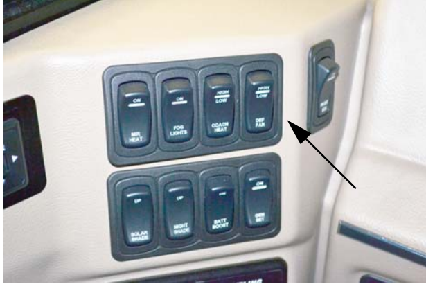
Defrost Fan Switch (Located on driver side dash) -Typical View
