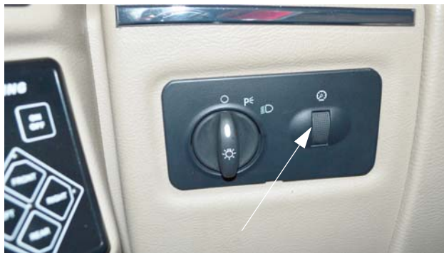
Driver Side Map Light Switch (Located on driver side dash)
