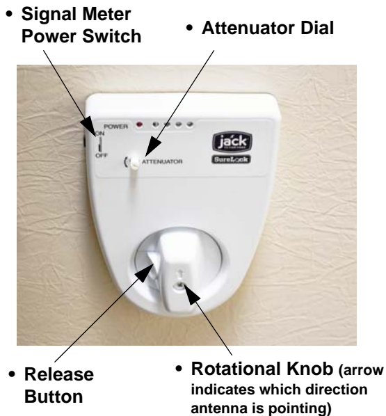
Digital Antenna Signal Meter (Located on ceiling)
