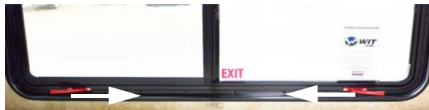
Escape Window (Pull both red safety latch handles inward and push window OUT) -Typical View
