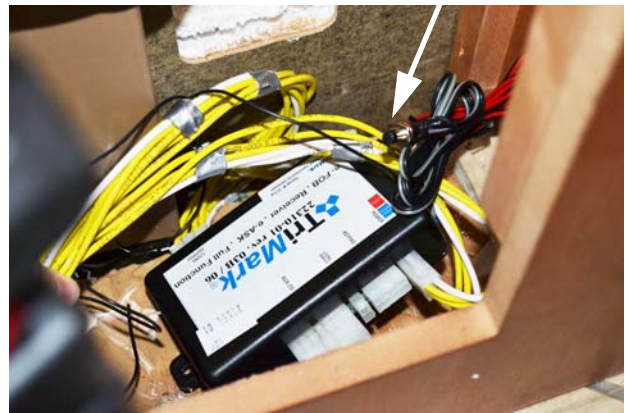
Keyless Entry Control Box (Located in passenger side trim panel. Remove magazine rack to access.) -Typical View
