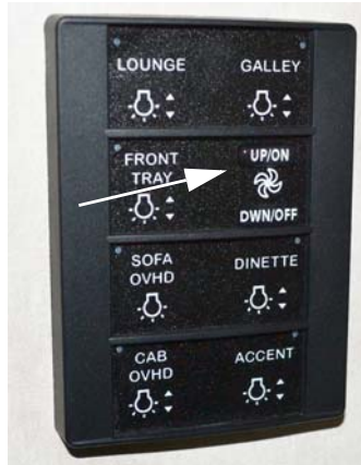
Power Roof Ventilator Switch
