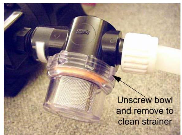
Water Pump Strainer -Typical View
