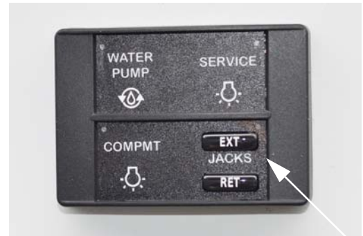
Auto Level Remote Switch (Located in the utility compartment) -Typical View
