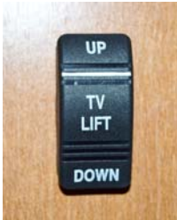
Buffet TV Power Lift/Lower Control Switch (Located on galley end near buffet)
