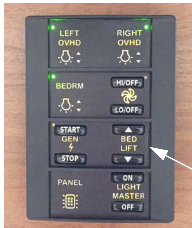
Power Lift/Lower Control Switch (Located on bed overhead cabinet or on a wall near the bed) -Typical View
