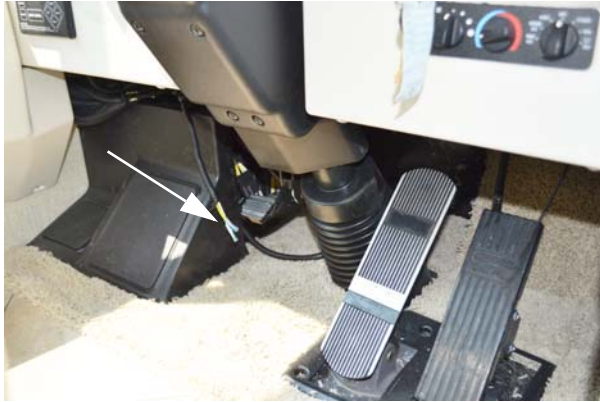
CB Power Wires -Typical View
