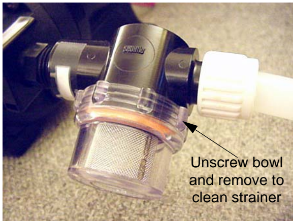
Water Pump Strainer -Typical View
