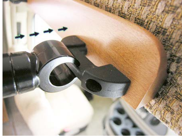
Attaching Bunk Ladder
