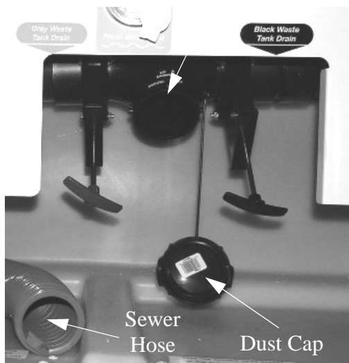
Holding Tank Dump Valves (Located in Water Service Center) -Typical View
