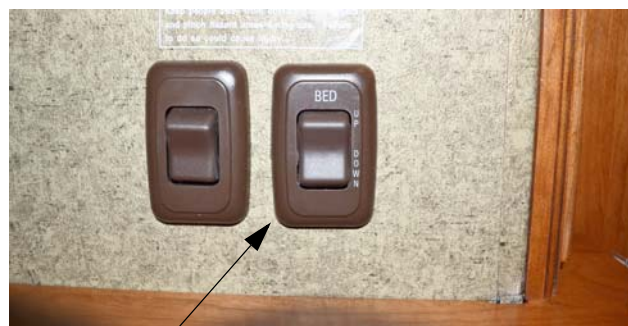
Power Lift/Lower Control Switch (Located near bedroom nightstand) -Typical View
