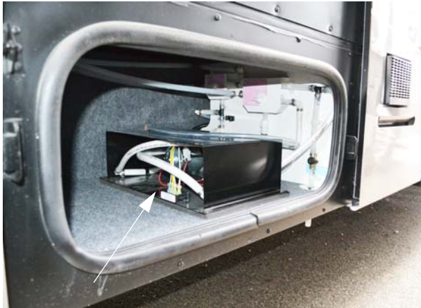
Water Pump (Located in compartment behind entrance door) * Model 35P shown
