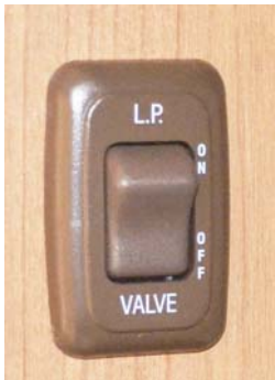
LP Tank Valve Switch
