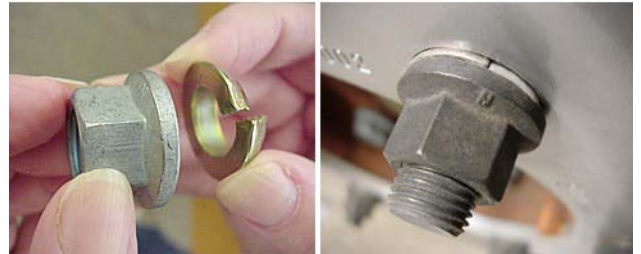
Steel Wheel Lug Nut and Washer (Hex Flange Nut with Split Cone Washer)
