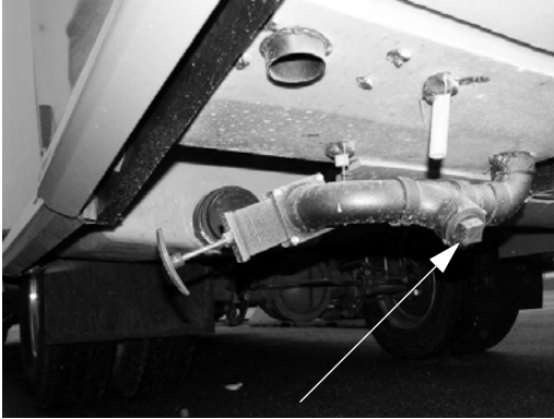
Waste Pump Drain (Located underneath rear driver side of coach) * Model 25T
