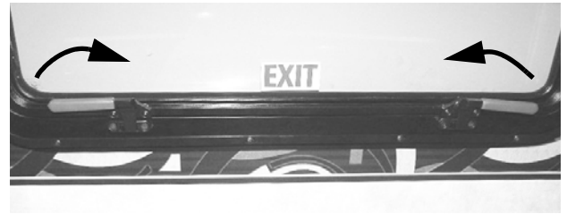
Escape Window (Lift both latch handles upward and push window open) -Typical View
