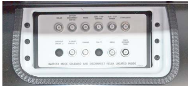
Automotive Chassis and House 12-Volt Circuit Breakers (Located in passenger side compartment)
