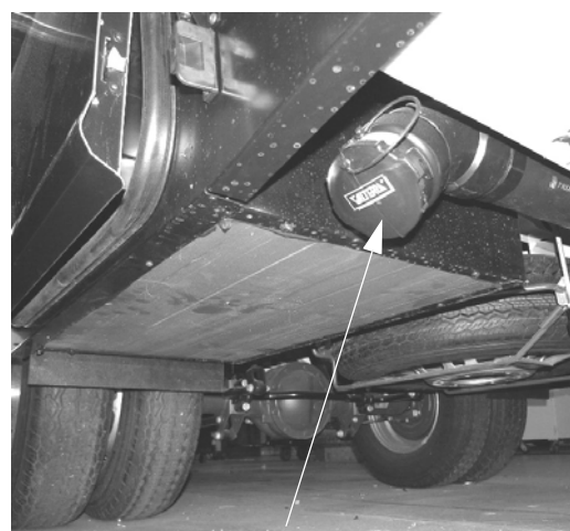
Sewage Drain Outlet (Located underneath coach behind driver side rear wheel) -Typical View
