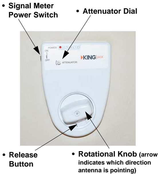
Digital Antenna Signal Meter (Located on ceiling)
