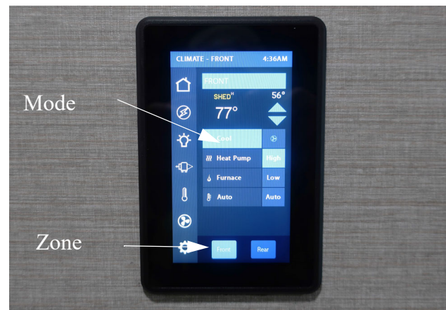
Thermostat “Climate” Screen (Located on Multiplex Monitor Panel)
