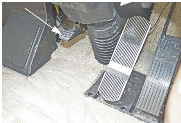
Press pedal down to adjust steering wheel tilt or telescope -Typical View
