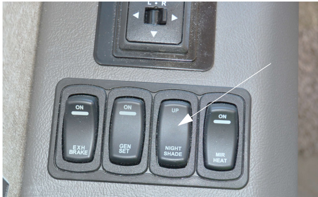
12-Volt Front Drop-Down Night Shade Switch (Located on driver side trim panel) -Typical View
