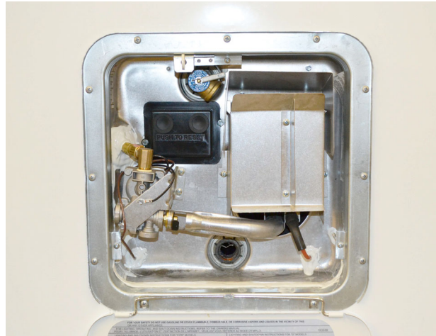
Water Heater Exterior Service Access
