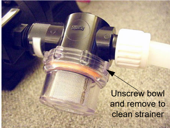
Water Pump Strainer -Typical View
