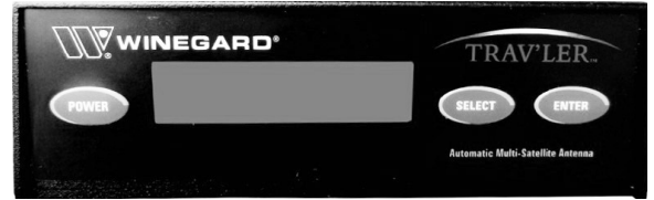
Automatic Multi-Satellite Dish Control (Located in overhead cabinet or entertainment center cabinet, depending on model) -Typical View
