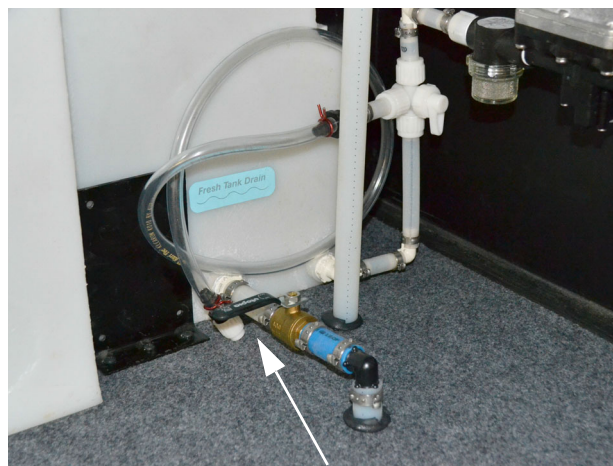
Water Tank Drain Valve (Located in passenger side compartment) *Model 38W shown
