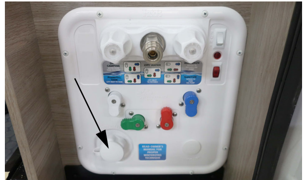
Tank Fill Inlet (Located behind the passenger rear door) -Typical View
