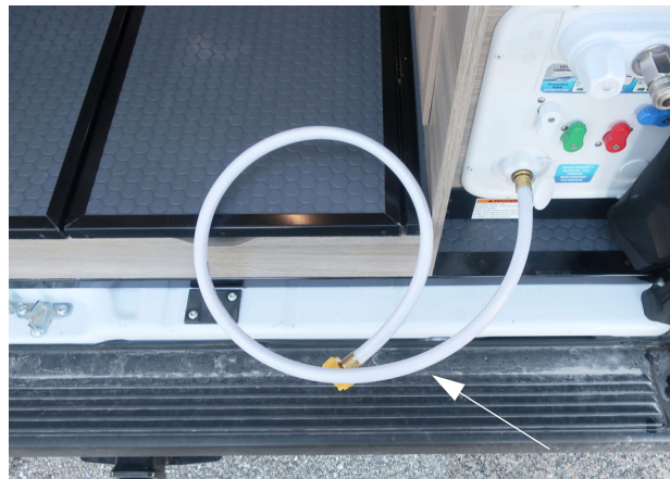
• Antifreeze Siphon Tube attached to the tank fill inlet -Typical View
