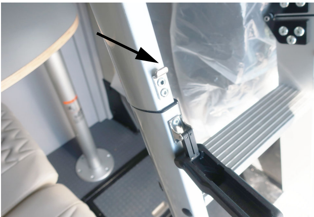
Hook that latch attaches to- the same on the right side -Typical View
