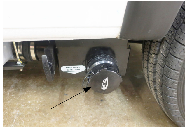
Sewage Drain Outlet (Located beneath motorhome) - Typical View
