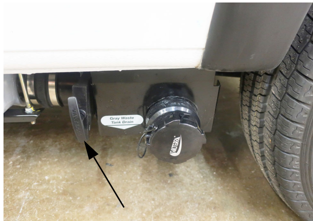
Gray waste tank drain valve (shown closed- pull lever out to drain) - Typical View
