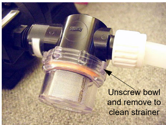
Water Pump Strainer -Typical View
