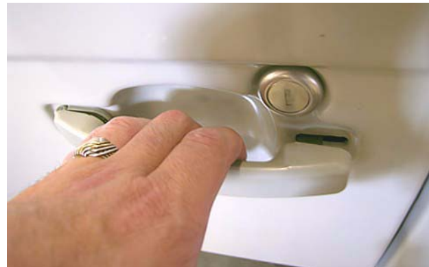
Pull door handles out to unlatch door
