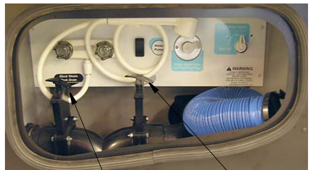
1st - Pull Black handle to drain Black Water (sewage) tank – then close.
