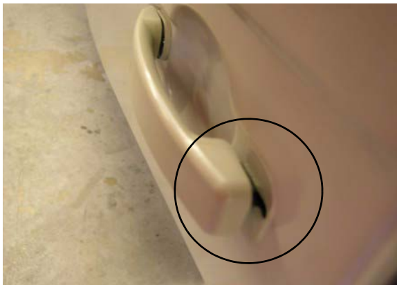
Door Unlatched (note gap)
