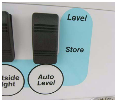
Auto Level Switch (Located inside Service Center compartment)
