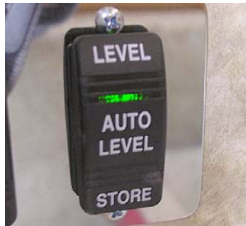
Auto Level Switch (Located inside entrance door)
