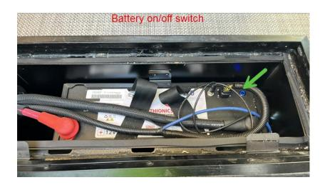
On units with the generator replacement the BMS is in the external front drivers side storage compartment.
