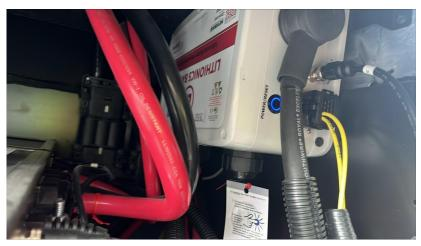
**6.** Turn off the chassis disconnect switch located above the gas pedal in the driver's foot well behind a removable plastic panel. Press the red button and pull out to disconnect the chassis battery.
