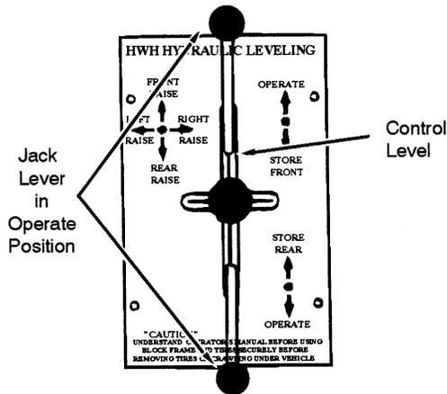
4. Swing the hydraulic jacks down by pushing the center Control Lever to Front Raise, then Rear Raise. A corresponding, red warning light will glow as each jack is in the vertical position.
