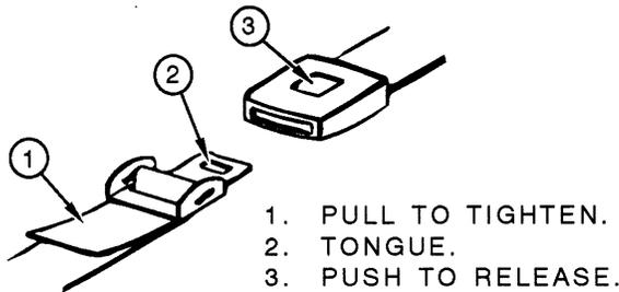
**Adjustment:** To lengthen belt, turn tongue at a right angle to belt and pull to desired length. To shorten, pull loose end of belt.
