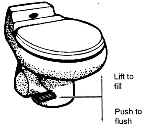
2. To flush the toilet, push the lever all the way down until sewage leaves the toilet and bowl is rinsed clean.
