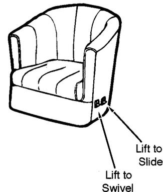
Swivel: Pull up on the swivel lever located on the side of the seat. The seat will lock into place whenever it reaches the center aisle facing position.
