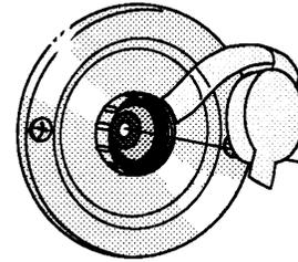
When connected to an outside source of water, the water bypasses the demand pump and storage tank and supplies pressure directly to individual faucets and toilet. A check valve built into the pump prevents water from entering the pump and filling the storage tank.
