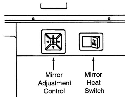
The power mirror control switch is intended for fine adjustment of the mirrors. If you cannot adjust a mirror properly using the control switch, it may need a coarse adjustment.
