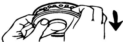
**Lowering Antenna to Travel Position** - Rotate antenna until pointer on rotating knob aligns with pointer on ceiling plate.
