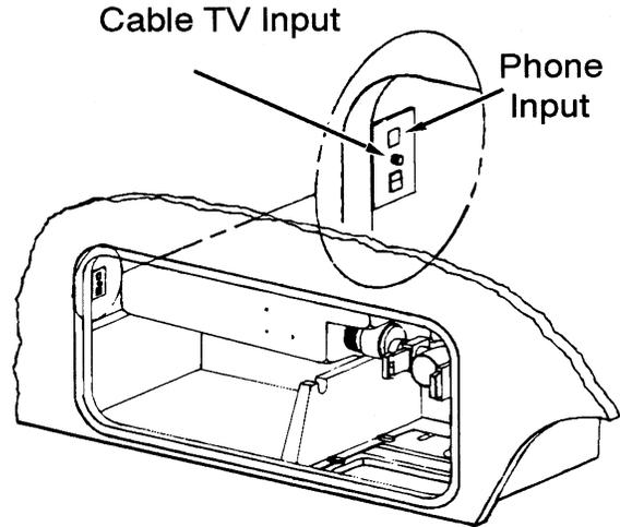
*NOTE: For coaches without the video control center option, be sure the TV antenna amplifier switch is turned OFF while connected to cable. The antenna amplifier will make the cable TV signal snowy.*
