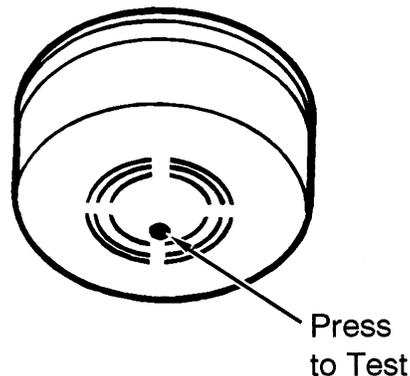
2. Your smoke alarm will not work without power. Never remove the battery to quiet the alarm. When your smoke alarm "beeps" about once a minute the battery is weak. Install a new battery immediately. Be sure to use only batteries specified in manual or on unit. Test unit after installing a new battery.
