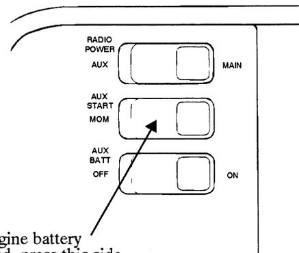
If engine battery is dead, press this side while turning ignition key for emergency starting power.
