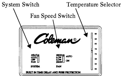
2. Slide thermostat switch from OFF to HEAT.
