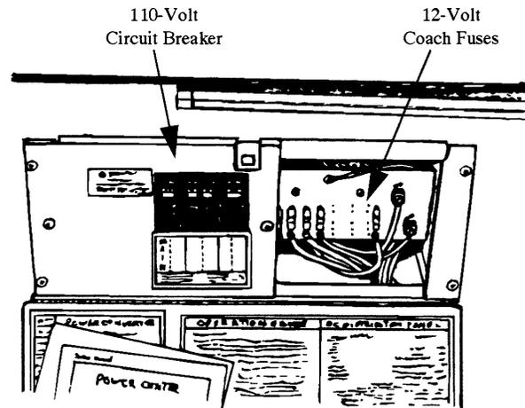
The fuse panel accepts only blade type plug-in fuses. Always replace fuses with those of the same amperage rating.
