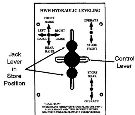
*NOTE: Coaches with the slide-out room option have vertical jacks that do not swing up. The jacks simply retract until they are in the stored position.*
