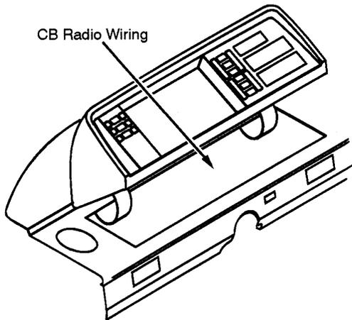
Look for a pair of wires, red and black, with connectors and flag labels, suspended from the wiring harness.
