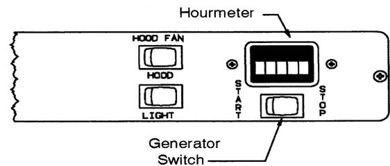
*NOTE: While the generator is running it is normal for the hourmeter to make a periodic "ticking" sound.*
