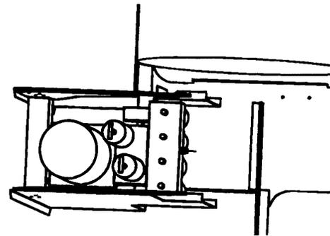
Hydraulic Pressure Release Valves viewed from center of vehicle.
