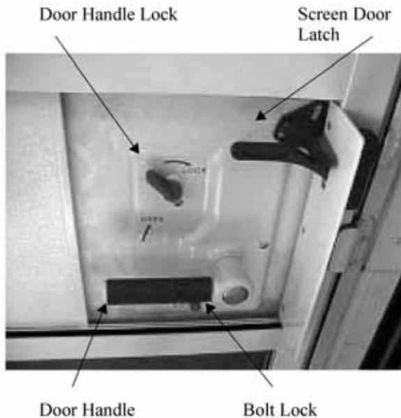
Lubricate the locks periodically with graphite to maintain good working condition.
