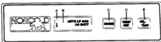
The ON/OFF button (E) turns the refrigerator On or Off. If the button is pressed, it will turn the refrigerator On and set the mode to AUTO. When the refrigerator is On, pressing this button for 2 seconds will turn the refrigerator Off.
