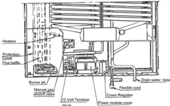
This refrigerator is equipped with an Automatic Energy Selector (AES) control system, which can automatically select the most suitable energy source which is available, either 120 Volt AC, or LP gas operation. The system can be set by the user to be fully automatic, or if desired, LP gas only. The refrigerator controls will work down to 9.6 volt DC.
