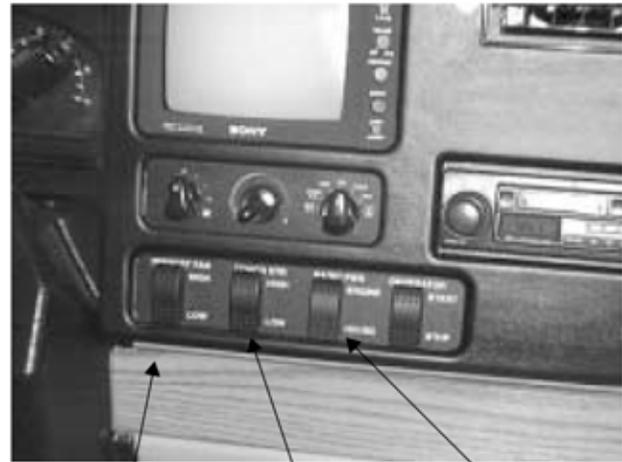
Windshield Defrost Fans      Rear Couch Heater Switch      Radio Power Switch
