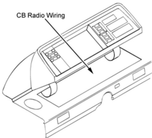
Look for a pair of wires, yellow (+) and white (-), with connectors and flag labels, suspended from the wiring harness.
