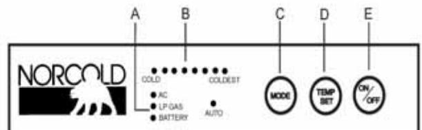
The On/Off button (E) turns the refrigerator On or OFF. When the refrigerator is Off, pressing this button will turn the refrigerator On and set the mode to AUTO. When the refrigerator is On, pressing this button for 2 seconds will turn the refrigerator Off.
