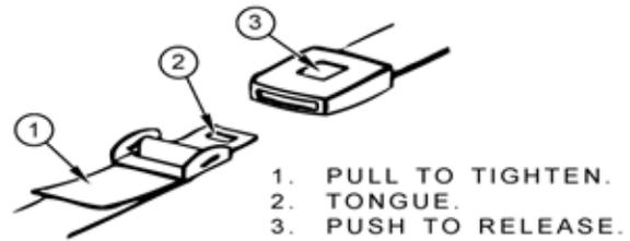
**Adjustment:** To lengthen belt, turn tongue at a right angle to belt and pull to desired length. To shorten, pull loose end of belt.
