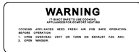
Unlike large homes, the oxygen supply inside a recreational vehicle is limited due to its size. To avoid danger of asphyxiation, provide proper ventilation when using the gas rangetop or gas oven. It is especially important not to use the gas oven and range top for comfort heating. Danger of asphyxiation is greater when these appliances are used for long periods of time without adequate ventilation.
