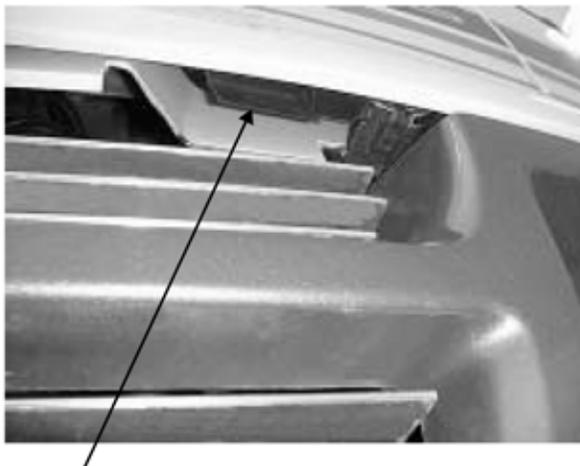
Squeeze latch handles toward hood panel and lower hood down into open position.
