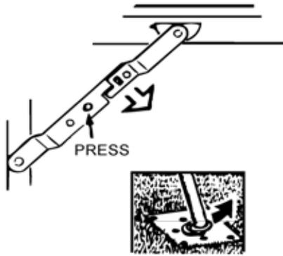
2. Remove the table from the wall support bracket by lifting the end of the table. Then lower the table to rest on the cleats attached to each dinette bench.
