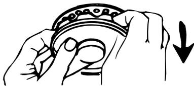
**Lowering Antenna to Travel Position** - Rotate antenna until pointer on rotating knob aligns with pointer on ceiling plate.
