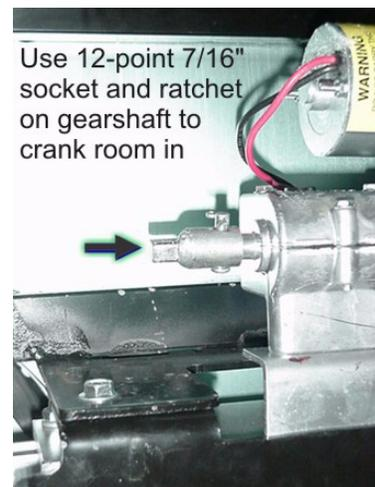
Use 12-point 7/16" socket and ratchet on gearshaft to crank room in
