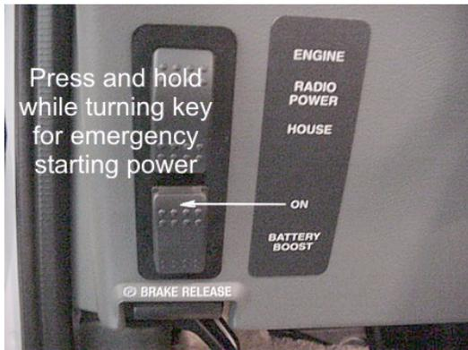
If engine battery is dead, press and hold while turning ignition key for emergency starting power.
