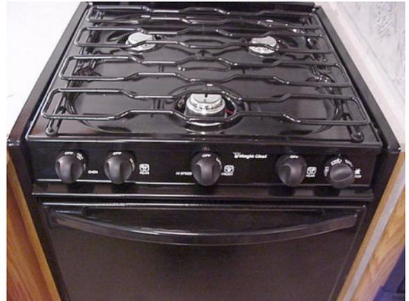
The range and oven in your motor home are operated on LP gas and will provide nearly all of the functions that the range in your home does. The range has a “Pilot Off” position on the oven control which allows the oven pilot to be turned off when traveling or refilling the LP tank.
