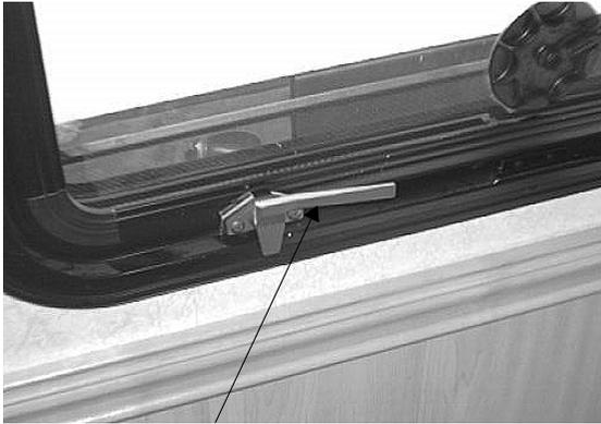
Lift latch handles upward to open.
