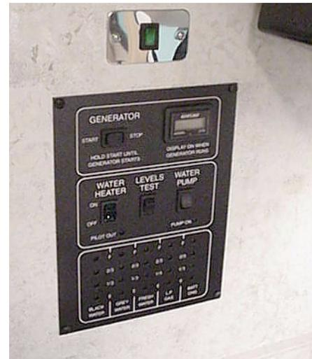
The Systems Monitor Panel provides a convenient central location for checking the condition of all utility systems in your coach. At the touch of a button this panel will display the fresh water and holding tank levels, LP gas tank level, plus the coach battery condition. You can start the auxiliary generator or turn on the water pump and water heater. Indicator lights tell you if the water pump is on or if the water heater pilot light is out.
