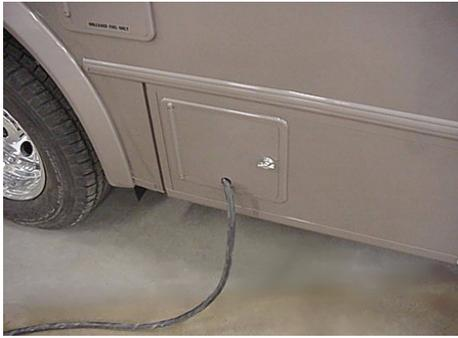
The three-prong power cord is designed to ground the electrical system through the receptacle. It is also designed to carry the amperage output of most campground outlets. If the electrical receptacle to be used is designed to mate with the three prongs on the power cord plug, the electrical connection can be expected to carry rated load. (See approximate power consumption table in this section.)
