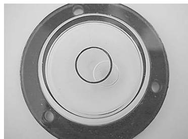
Normal vehicle leveling to provide comfort for the occupants is satisfactory for refrigerator operation. This will be well within the operation limits of 3° off-level side-to-side and 6° off-level front-to-back.
