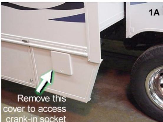
Remove this cover to access crank-in socket
