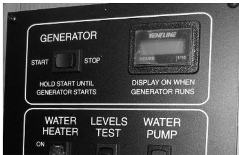
Generator Switch and Hourmeter on monitor panel
