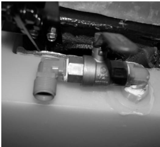
**Water Tank Drain Valve**
