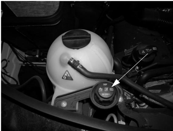
Diesel Exhaust Fluid Fill
