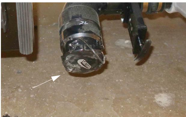
**Sewage Drain Outlet/Dust Cap**
