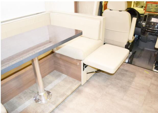
2. **To Store:** Push in levers to release locking arms and lower into the stored position.
