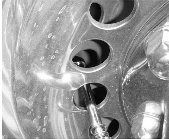
6. When tire pressure testing is complete, reinstall the valve stem cap (with the cap still retained in the valve cap tool end).
