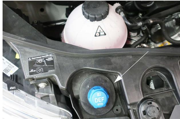
Diesel Exhaust Fluid Fill
