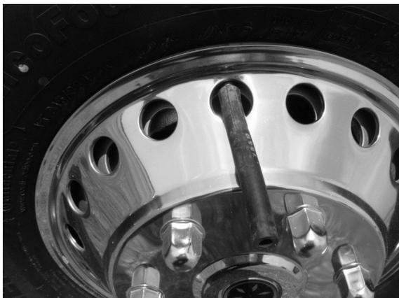
4. Using the valve cap tool as a remote handle, unscrew the valve stem cap (retaining cap in the end of the valve cap tool).
