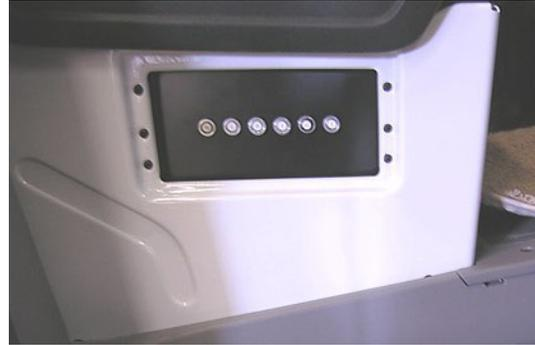
Automotive Chassis 12-Volt Circuit Breakers
