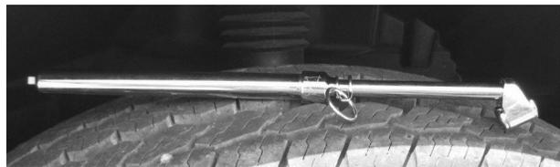
2. To check rear outer dual tire pressure, use the long handle of the tire gauge to control alignment on the fill-through extension.
