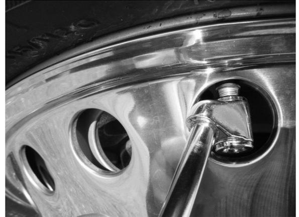
6. When tire pressure testing is complete, reinstall the valve stem cap (with the cap still retained in the valve cap tool end).
