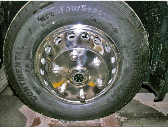
The wheel on your motorhome has a push on liner which is removed similar to a hubcap. Remove the covers by carefully prying the perimeter flange away from the wheel flange.
