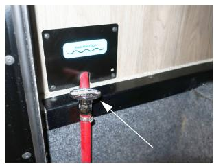
Open the Tailgate Drain Valve (Model 622A)
