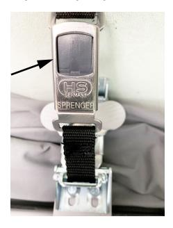
Locate the retention clamps on the driver's and passenger's side of the Pop-Top, and push the black button to release.
