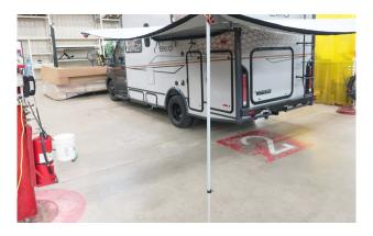
•Extend the support leg downward. The leg can be adjusted for height. Reverse the steps to place the awning back into travel configuration. -Typical View
