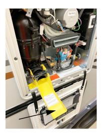
Water heater Easy Drain Lever in lowered position.
