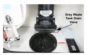
Sewage Drain outlet (Located inside the service center on the drivers side) -Typical View
