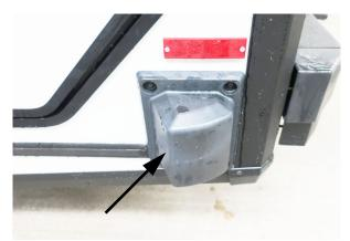
Driver side blind spot sensor location. Do not paint or cover this block.
