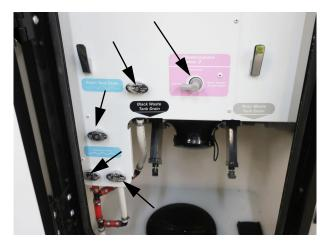
Waterlines and Tank Drain Valves (Shown in the closed position)
