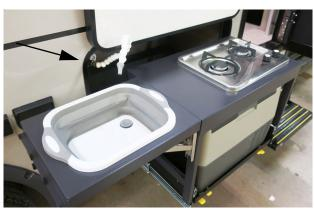
Faucet shown installed. The segmented faucet can be bent and turned to the desired position.
