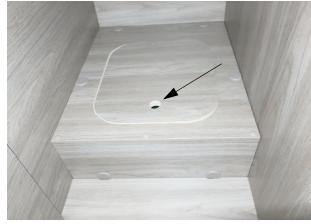
• To access the water pump strainer, first locate the hole in the passenger side bed lower forward storage area.
