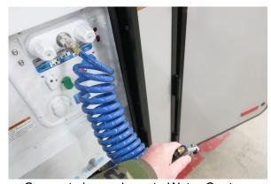
Connect shower hose to Water Center Panel faucet (Located inside the service compartment), then squeeze handle until water stops flowing. Do this for the exterior wash station located in the exterior kitchen compartment also.
