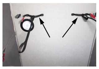
Press up firmly on the handles and lift the Pop-Top until the shocks take over and extend the Pop-Top to the extended position.
