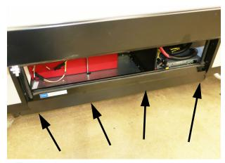
The 4 screws to remove the retention panel are located on the bottom.
