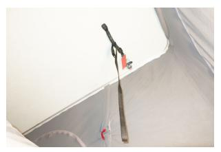
Reverse the steps to collapse the Pop-Top into the travel position. Use the straps that are attached to the handles to assist pulling the Pop-Top down. The red tab handles located on the sides are designed to pull the material inward, to ensure that the Pop-Top does not close down and pinch itself.
