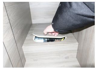
Lift up on the access panel to expose the water pump.
