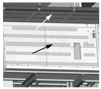
A cut away drawing with the back wall removed. The brackets run horizontal on the inside wall and on the ceiling. Shown in darker shades. These are not visible. Locate these brackets using a magnet.
