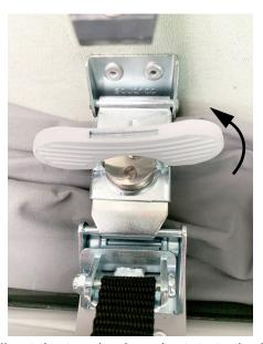
Pull out the turn knob and rotate to the left until the latch is extended.
