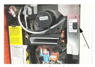
Water Heater Power Switch (Located behind water heater access panel on exterior of the motorhome) -Typical View
