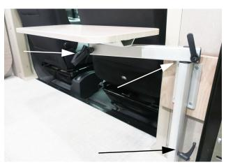
There are 3 adjustment levers that alter the height, length, and position of the table.
