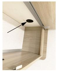
Roof Access Port (Located inside rear overhead cabinet). -Typical View
