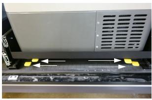
• Push the yellow tabs outward to release and slide out the tailgate package. The upper tabs release the refrigerator, while the lower tabs release the stove and sink package.
