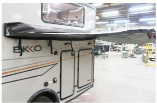
•On the end closest to the drivers side, pull the awning outward and it will reach around to the backside of the motorhome.
