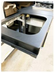
•The tailgate package also comes with a removable sink attachment. To install, lift up the sink table until it locks into place.
