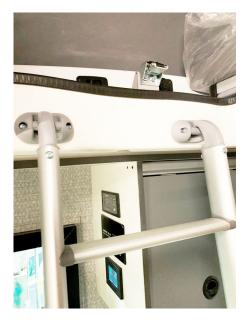
Attach the ladder to the attachment points located on the passenger side. The ladder hooks in from the top.
