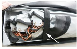
After unzipping and exposing awning, release the velcro retention straps.
