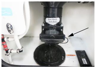
Sewage Drain Outlet with drain valve (Located inside the service center on the drivers side pull valve outward to open)
