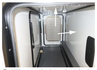
The hidden support brackets are located on the wall and the ceiling in the Gear Garage. (Use a magnet to locate.)
