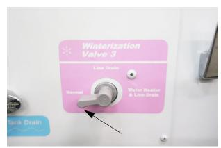
Place the Winterization Valve 3 into the "Normal" position.
