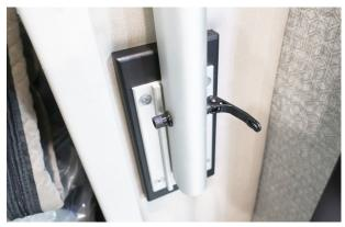
The attachment point is located inside the passengers wall next to the main entry door.
