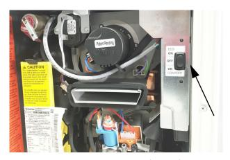
Water Heater switch located behind the water heater access panel of the exterior of the motor home.
