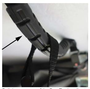
Pull down on one of the Pop-Top handles to create slack to release the latch. Follow these steps to release the driver's and the passenger's side.
