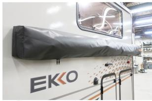
• The manual awning is located on the drivers side rear of the motorhome. Start by unzipping the awning. The awning case remain permanently attached to the side of the motorhome.
