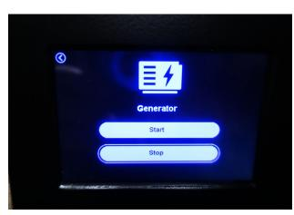
Select the Generator Icon on the main menu to access the Generator start/stop screen.
