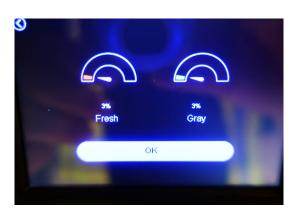
Select the Tank Level icon on the main menu to view the Fresh Water and Gray tank levels screen.
