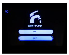
Select the Water Pump icon on the main menu to access the water pump ON/OFF button. -Typical View
