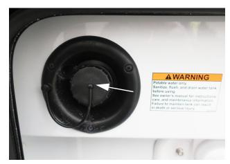
Water Tank Gravity Fill (Located in the water center)
