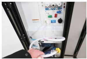
Attach a siphon tube then place it in the chlorine solution container and turn the pump on to begin siphoning contents.
