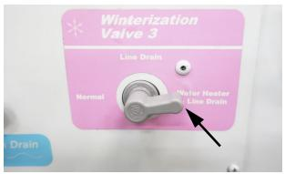
Winterization Valve 3 turned to the "Water Heater and Line Drain" position.
