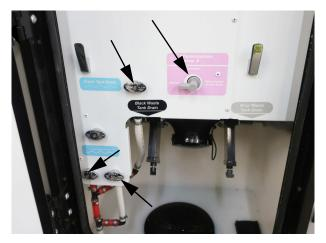
Open the Waterlines and Tank Drain Valves indicated by the arrows.
