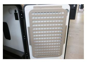
MOLLE Panel on the Passenger side Gear Garage access door. -Typical View
