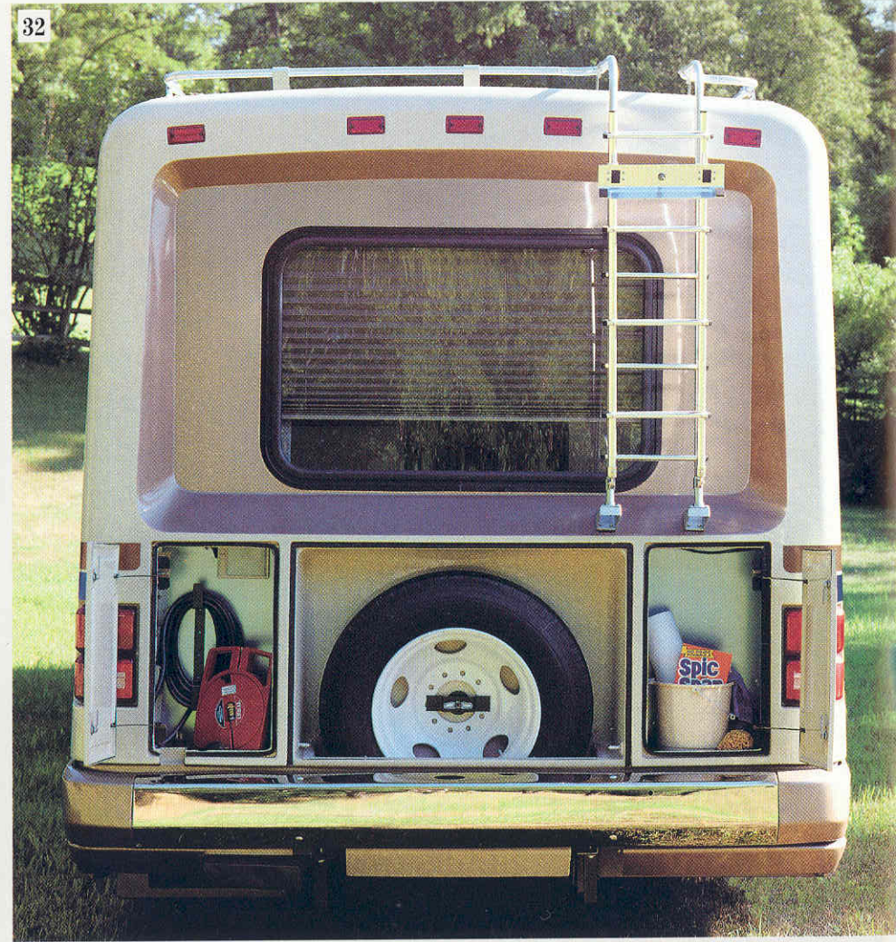
29. The storage bays are wide and roomy and the two deep-cycle batteries pull out of a separate storage bay for easy access. 30. For excellent accessibility the storage compartment doors feature spring-loaded door holders. There is also a 57" deep compartment for carrying longer items. 31. The single-piece rear cap provides an attractive finish for the separate insulated inner rear wall. 32. The rear cap has three compartments: one for your own odds and ends; one for the spare tire; and a lighted compartment for the electrical cord, cable TV hookup and garden hose/reel. 33. The handsome 23RC gives you Chieftain's high storage in a short
